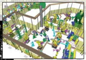
Production environment optimised using DELMIA.
